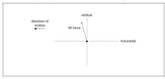
Draw the forces acting on the glider to complete the free-body diagram. The dotted lines show the horizontal and vertical directions.
