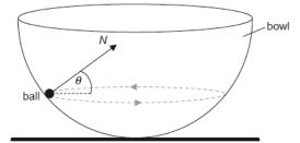
The normal reaction force *N* makes an angle  $\theta$  to the horizontal.
