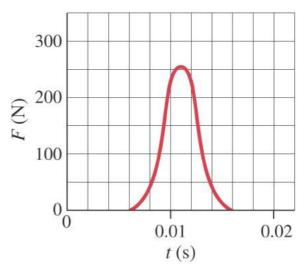
(a) The impulse given the ball is the area under the F vs. t graph. Approximate the area as a triangle of "height" 250 N, and "width" 0.01 sec.
