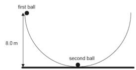
The first ball is released and eventually strikes the second ball. The two balls remain in contact. Determine, in m, the maximum height reached by the two balls.
