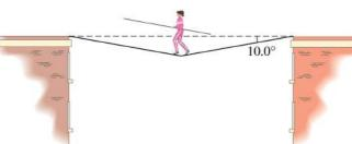
Consider the point in the rope directly below Arlene. That point can be analyzed as having three forces on it – Arlene's weight, the tension in the rope towards the right point of connection, and the tension in the rope towards the left point of connection. Assuming the rope is massless, those two tensions will be of the same
