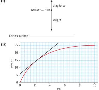
the acceleration of the ball is equal to the gradient of the graph gradient =  $\frac{25-6}{4.8-0}$  $= 4.0 \text{ m s}^{-2}$
