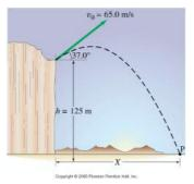
Choose the origin to be at ground level, under the place where the projectile is launched, and upwards to be the positive y direction. For the projectile,  $v_0 = 65.0 \text{ m/s}$ ,  $\theta_0 = 37.0^\circ$ ,  $a_y = -g$ ,
